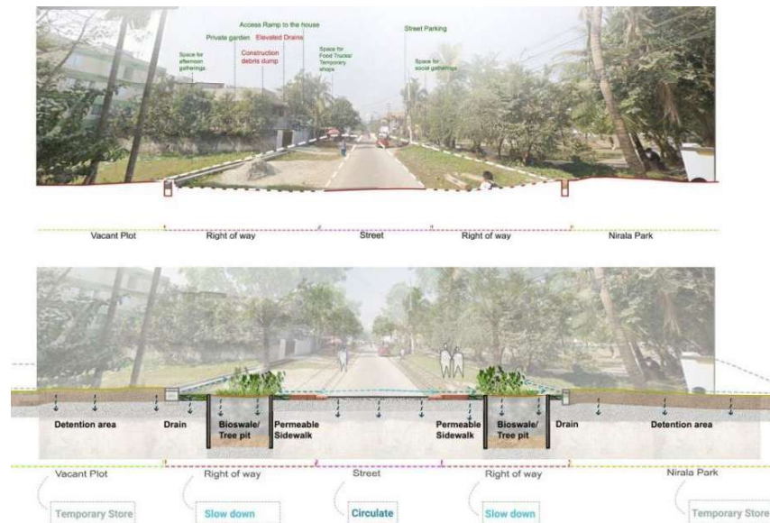
Figure 5. Potential spatial organizations and types of green infrastructures to slow down, circulate, recharge into the ground, and store in possible locations in the interstitial “Third Landscapes” at the street scale. Diagram by the author. Background image: Google Street View.
