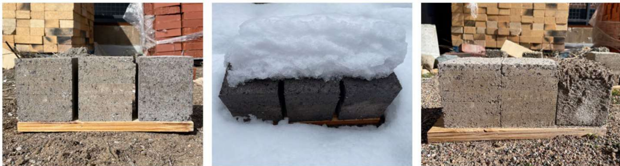
Figure 1. Sample experiment documentation. This student left samples outside over a period of 8 weeks to understand the impact of precipitation and freeze/thaw on material durability. Work found that the samples with a low percentage of clay and no cement degraded quickly. Student work.
