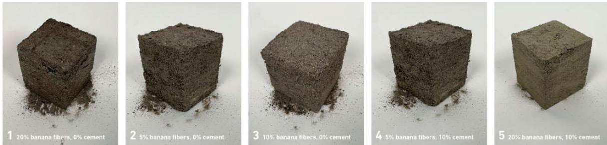
Figure 2. Five material samples reinforced with banana fibers, with cement content ranging from 0% to 10%. Mix proportions varied from 20% fibers (Sample 1) to 5% fibers (Sample 5). Student work.
